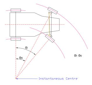
Figure 2.4: Inclined track-rod arms giving true rolling in three positions.
