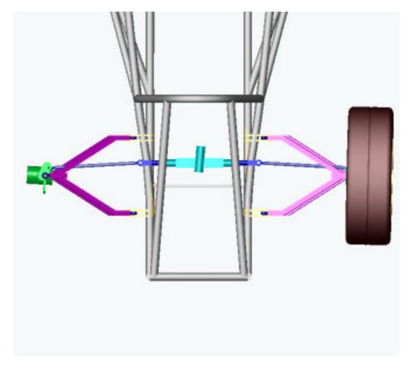
Figure 7.2: Final model of the steering system.
