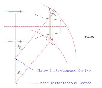
Figure 2.3: Parallel track-rod arms giving true rolling at straight ahead only.
