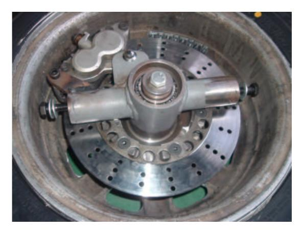
Figure B.3: Front upright mounted in road wheel.
