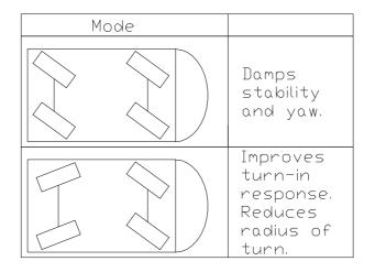
Figure 2.10: The effects of the two modes of the Nissan HICAS steering system.
