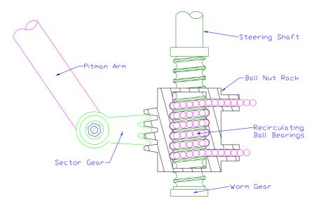
Figure 2.15: Recirculating ball steering box.
