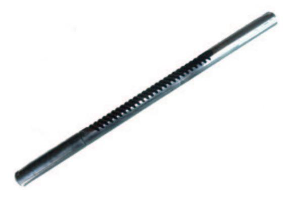
Figure 4.2: Renault R10 rack after modification.
