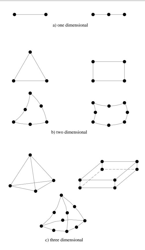
Figure 1.1: Common finite elements.
