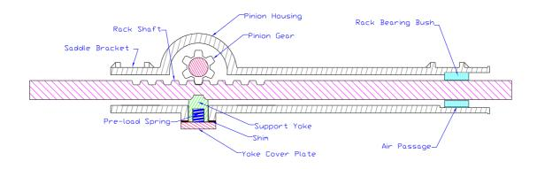
Figure 2.11: Rack and pinion steering box.
