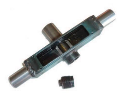
Figure 4.3: Complete housing for modified rack and pinion.
