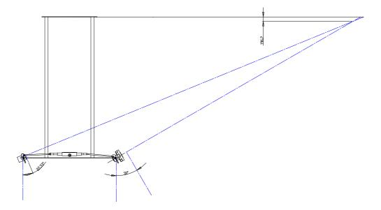
Figure 7.1: Model showing inside wheel at 30 degrees. Note also steering box location 50mm behind front axle line.
