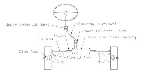
Figure 2.12: Rack and pinion steering linkage.
