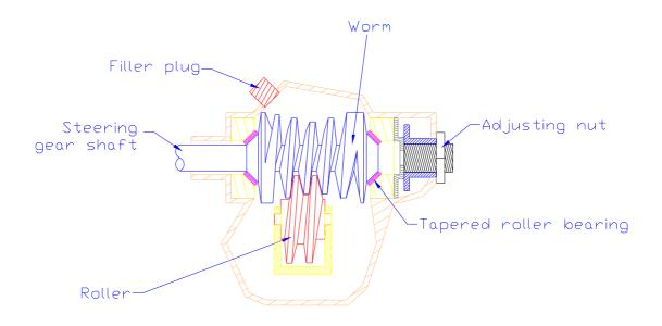
Figure 2.17: Worm and roller steering box.
