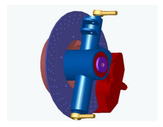
Figure 5.8: Model of final stub axle assembly.
