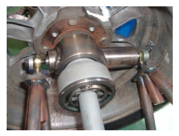
Figure B.5: Rear upright mounted in road wheel and suspension arms.
