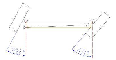
Figure 2.5: Outer wheel turns at a greater angle than the inner wheel.
