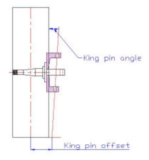
Figure 3.1: King pin angle and offset.
