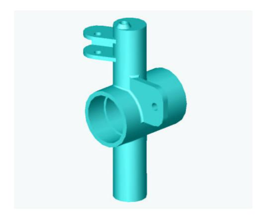
Figure 5.11: Right view of final model of left upright.
