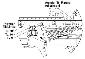
**Figure 10.41:** *Anterior tilt range adjustment*
