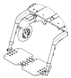
Figure 10.9: Interlocking angle adjustable footplate
