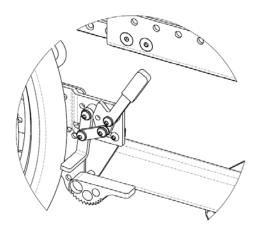
Figure 10.26: Wheel Lock with Anti-Rollback Device
