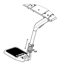
Figure 10.4: Adjusting mount height
