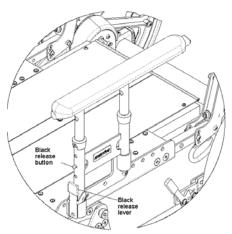
Figure 10.10: Adjusting armrest height for dual post
