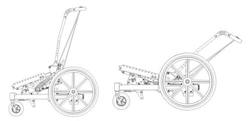
Figure 10.33: Dynamic backrest recline in combination with tilt
