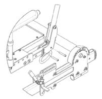
**Figure 10.15:** Adjusting the back angle for non-fold down backrest
