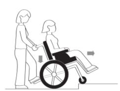
**Figure 3.1:** Assistant positioning for climbing curbs, for wheelchair with step tubes
