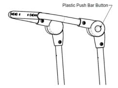
Figure 10.37: Adjustable push bar handle
