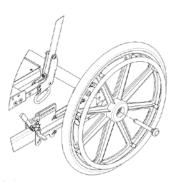
**Figure 10.17:** Removing rear wheels fastened with quick release axle.
