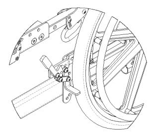
Figure 10.22: Push to Lock Wheel Locks (Standard)
