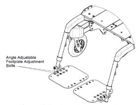
Figure 10.6: Adjustable angle footplates
