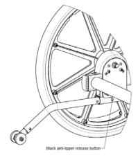
**Figure 10.19:** *Installing anti-tip tubes*
