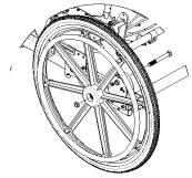
Figure 10.16: Removing rear wheels fastened with axle bolt.
