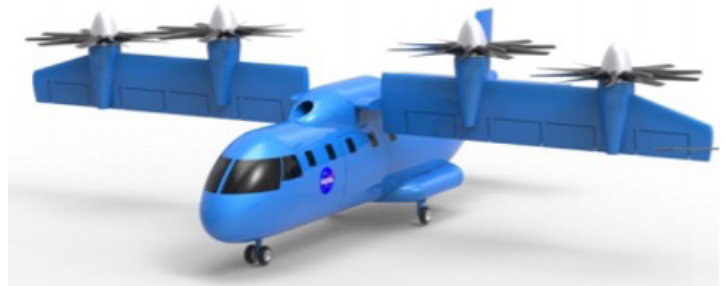
Figure 3. On some aircraft, the propellers can rotate to provide upward lift or forward thrust. Credit: NASA
