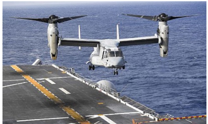
Figure 6. The V-22 Osprey can tilt its rotors up for takeoff and landing. Credit: U.S. Navy photo by Mass Communication Specialist 3rd Class Vincent E. Zline
