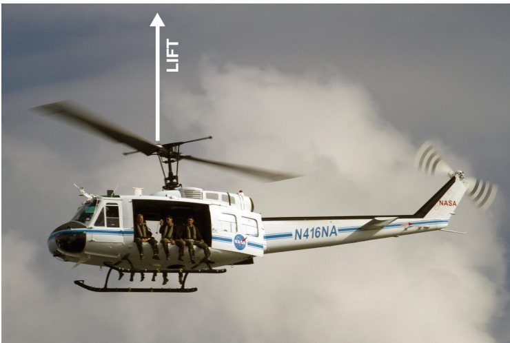
Figure 1. The blades on a helicopter create lift that moves it upward. Credit: NASA/ Dan Casper
