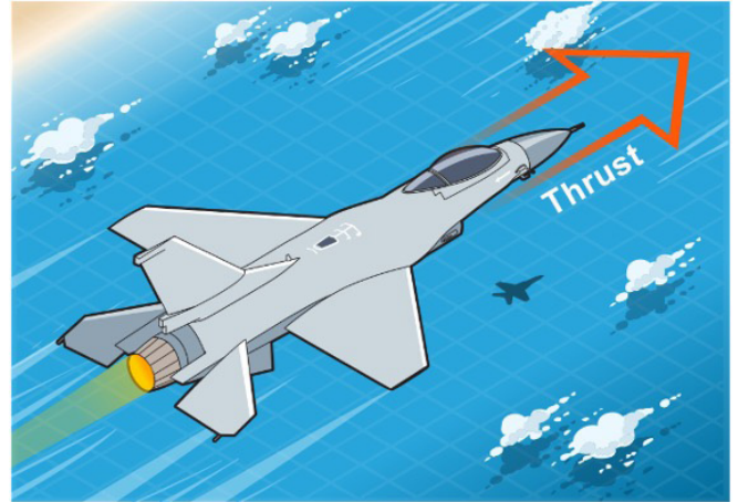
Figure 5. Hot gases coming out the back of a jet create thrust. Credit: NASA
