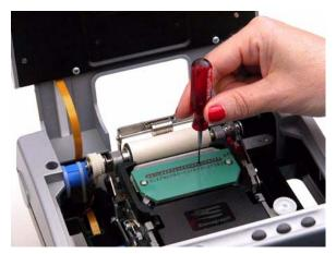
Adjust the number bar contact only when <u>all</u> your number settings are either too heavy or too light. To adjust an individual number, adjust the contact of the corresponding letter for that number. For example, to adjust the number 8, adjust the key contact for the final L. By adjusting the number 8, you also adjust the letter L.
