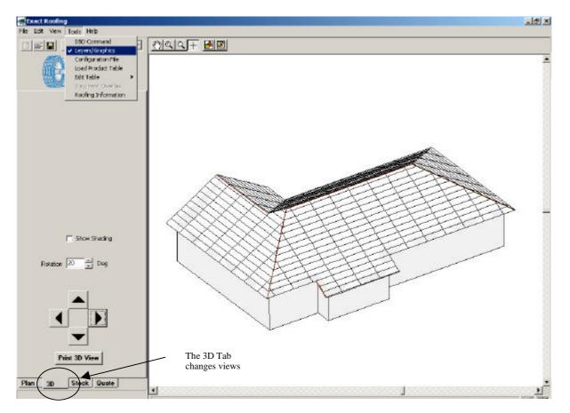
The 3D diagram can be rotated (by default 20 degrees at a time) and the user can verify the house was drawn correctly.
