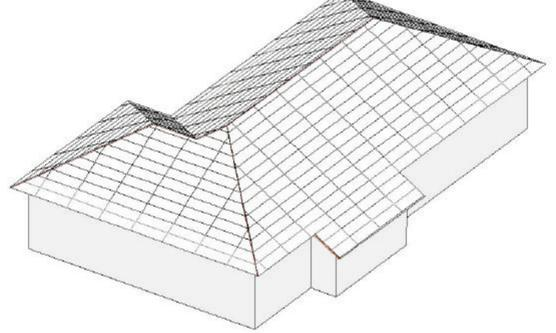
Begin by drawing the outline of the roof. Enter from the pull down menu **Plan->Construct->Outline** as shown below:
