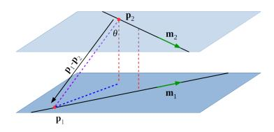
The normal to the two planes is given by  $\mathbf{m}_1 \times \mathbf{m}_2$ , and a unit vector in this direction is  $(\mathbf{m}_1 \times \mathbf{m}_2)$
