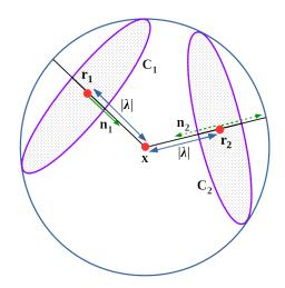
The position of the centre of the sphere will be given by  $\mathbf{r_2} \pm \lambda \mathbf{n_2}$ , where the sign will depend on the direction of  $\mathbf{n_2}$  and sign of  $\lambda$ .
