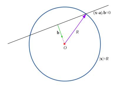
For the plane and sphere to intersect we need to have the perpendicular distance of the plane from the origin to be less than R.
