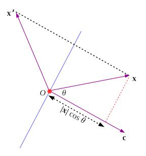
From this we can see that  $\mathbf{x}'$  is the reflection of vector  $\mathbf{x}$  in the plane through the origin with perpendicular vector  $\mathbf{c}$ .
