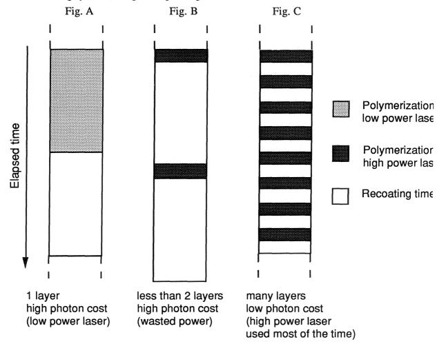
Fig. A shows that a small laser is properly dimensioned in the historical first generation SPL technology. One could therefore say that, given the current artificial constraints, first generation machinery is <u>properly</u> (not efficiently) defined.
