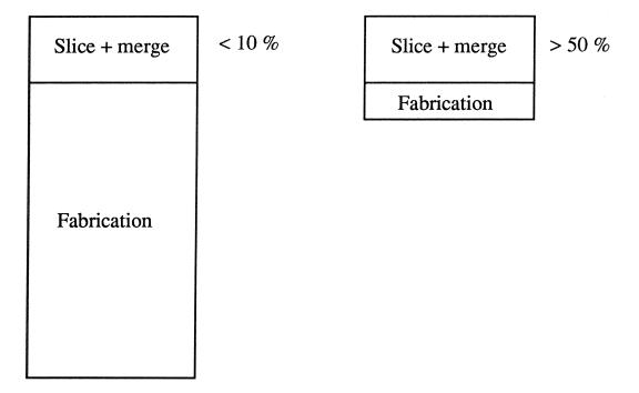
Therefore, if one wants to take advantage of a powerful laser, one must also define a new manufacturing strategy, where the new bottlenecks are properly managed. One must improve all manufacturing sequences by at least the same efficiency factors as the expensive increase in laser power. This imposed very substantial new SPL software design, and explains the reason why the second generation SPL 1000 /LSA is using <u>much more powerful</u> computers than the first generation SPL systems.
