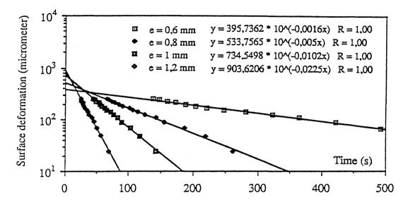
FIG. 1: Surface relaxation versus time for different layer thickness (e)
