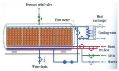
Fig. 6.5 Water spray or cascading water retort
