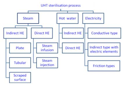
Fig. 6.9 Classification of UHT sterilization process
