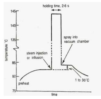
Direct heating injection type system
