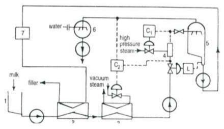
Fig. 6.13 UHT sterilization process (direct heating type)
