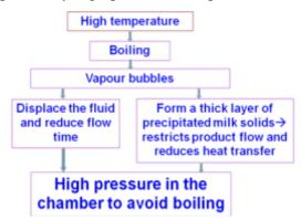
Fig. 6.11 Why high pressure is required in chambers
