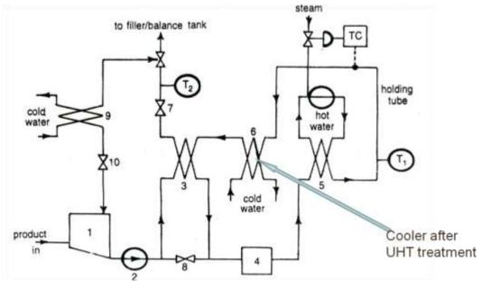
Fig. 6.10 UHT sterilization process (indirect heating type)
