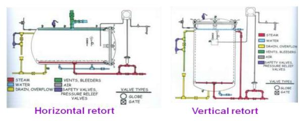
Fig. 6.4 Basic parts of retort
