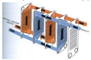
Fig. 6.12 Schematic diagram of a plate heat exchanger
