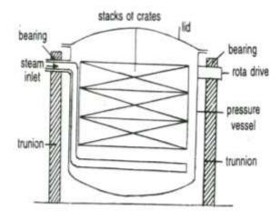
Fig. 6.6 Rotary batch sterilizer
