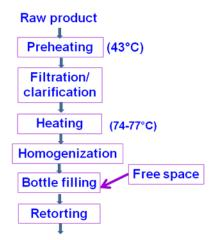
Fig. 6.2 In-bottle sterilization process
