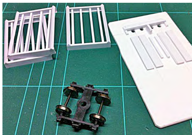
Cane trucks: the frames (upper left) are assembled using the jig (right). Mounting the frames on low profile Bachmann trucks eliminates the need to build carefully engineered bearing mounts, etc.
