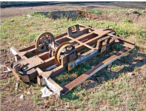
FSC standard steel cane trucks showing deck structure (top) and underframe details (below). Lautoka Mill, 2007.
