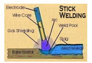
Another confusing concept concerns polarity in welding. Notice in the two charts shown earlier that there are three choices available under "Current". AC represents the familiar alternating current, which is an acceptable option for all the electrodes listed there, except E-6010. The other two options, which pertain to DC (direct current), require a little explanation.
