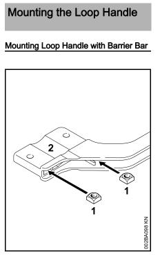
• Fit the square nuts (1) in the barrier bar (2); the holes must line up.
