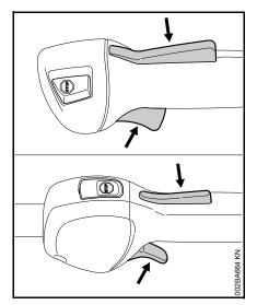
Press down the throttle trigger lockout and open the throttle – the choke knob moves to the run position I. After a cold start, warm up the engine by opening the throttle several times.
