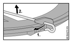
Disconnect wire rod from the transport guard.
