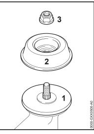
Depending on the cutting attachment, it may be necessary to use the nut (3) and rider plate (2). The thrust plate (1) must be used with all cutting attachments.
