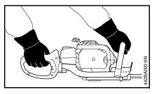
Right hand on the control handle and left hand on the front handle.
