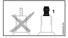
If the spark plug comes with a detachable adapter nut (1), screw the adapter onto the thread and tighten it down **firmly** to reduce the **risk of arcing and fire**.
