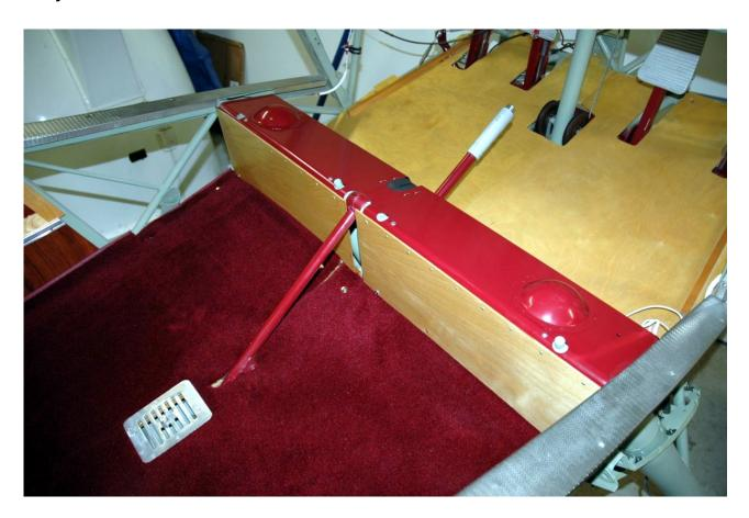
Access to the shock struts is gained by removing the shock tower cover. Remove the seats first, then remove the screws along the front and back of the cover.
