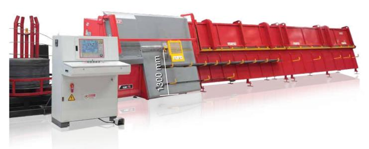
**PLANET F13** allows to get coplanar shapes and stirrups continuously closed, eliminating the dangerous manual operator intervention during the bending phase.
