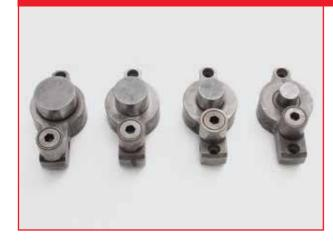
PLANET F13 is equipped with a series of monobloc bending pins at quick fixation, which allow a fast production restart at each wire change diameter.
