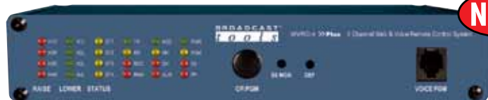
WVRC-4 Plus 4 Channel Web & Voice Remote Control System
