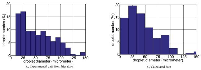
Fig. 3 Comparison of experimental [21] and calculated data of the initial droplet size distributions. The impeller speed was 350 rpm, the dispersed phase volume fraction was 0.3.
