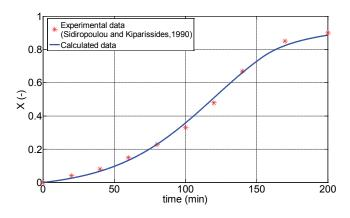
Fig. 2 The time profiles of experimental data from literature and simulation data. The droplet size distribution was uniform, all droplets contained the same amount of initiator, the amount of initiator was 0.0029 mole % based on monomer and the temperature was 323.
