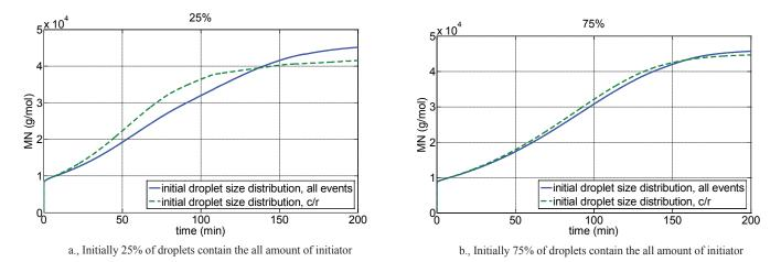
Fig. 7 The effect of meso-scale interactions on number average molecular weight, initially 25% of droplets contain initiator. The amount of initiator was 0.0029 mole % based on monomer and the continuous phase temperature was 323 K
