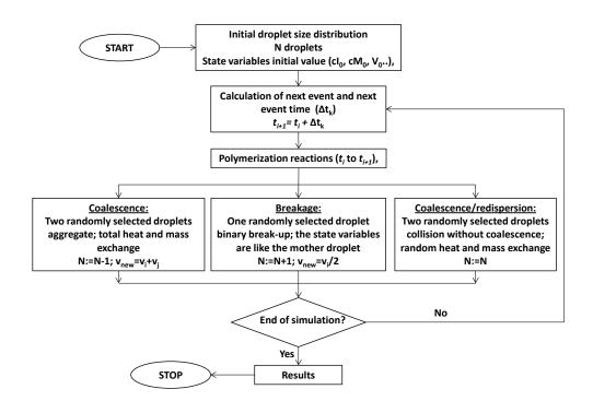
Fig. 1 Algorithm of coupled continuous time - Monte Carlo method
