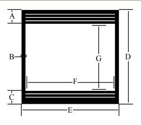
Measurement A is measured from the top of the exposed black metal, down to the top of the fireplace opening.
