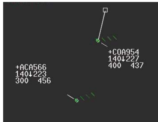
Figure 6 - Full data blocks. ACA566 and COA954 display the usual full datablock. COA954 also displays a TACT MDM.
