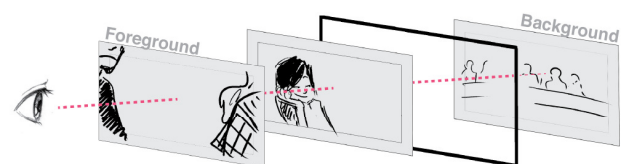
Figure 4. Illustration of our approach: stereoscopic 3D planes are stacked to form the middle image of Figure 1.
