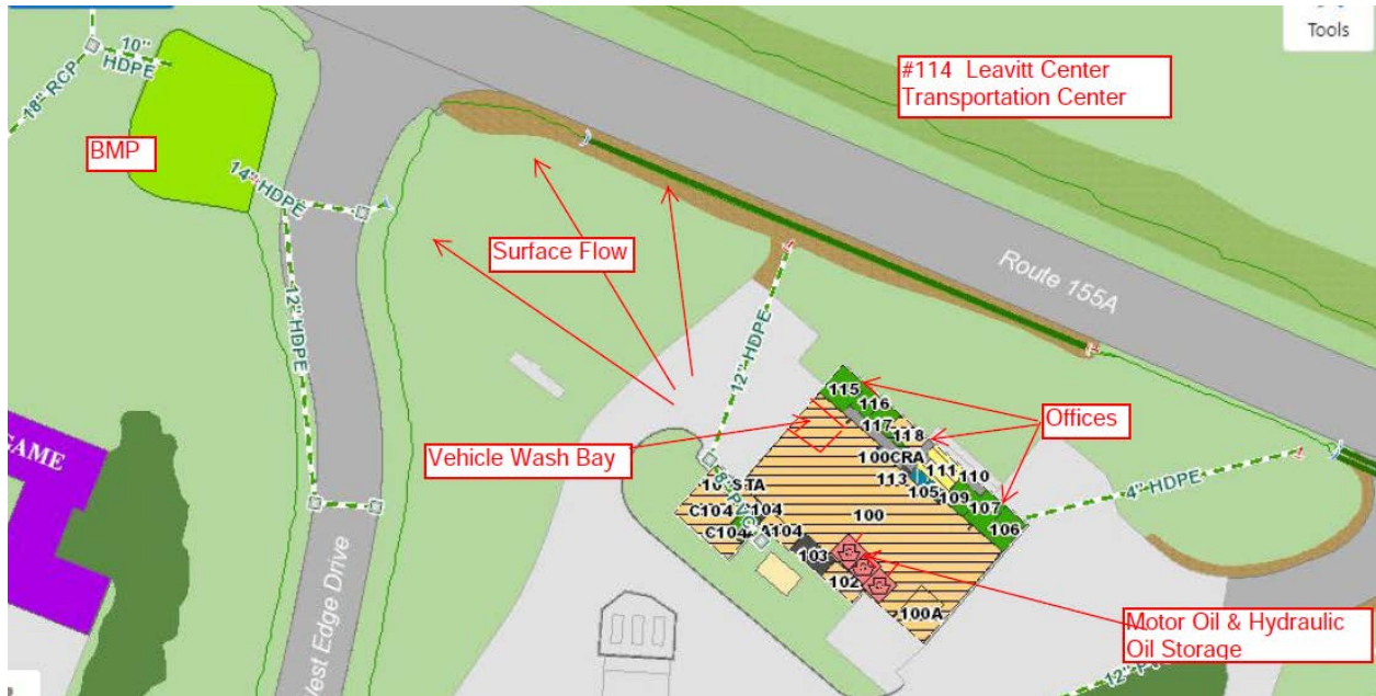
Attachment 1: Facility site map identifying key buildings and sites, the location of all known floor drains that tie into the stormwater drainage system, stormwater outfalls, and their receiving waters.
