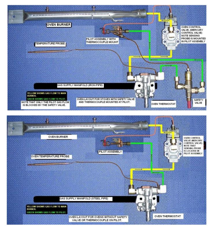
All Seaward / Princess / Hillerange stoves built after about 1993 should have an oven thermocouple & safety valve. Stoves built between 1984 & 1993 might have an oven thermocouple & safety valve.
