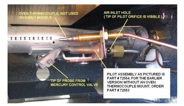
If the main burner does come on when extra heat is added, the pilot flame PROBABLY just isn't getting the probe hot enough. (Again, look for dirty pilot orifice, bent pilot assembly, low gas pressure.) Verify the probe is properly located in the pilot assembly.
