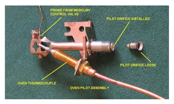
If you have the thermostat turned up, and the pilot size is big, and you apply additional heat to the probe but the main burner still won't light, you probably have a defective mercury control valve.
