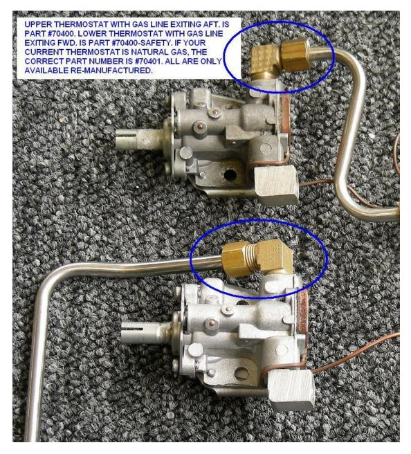
The #70400 ( CNG version is #70401 ) can be identified by the "triangularish" shaped copper plate attached to the rear of the thermostat body.
