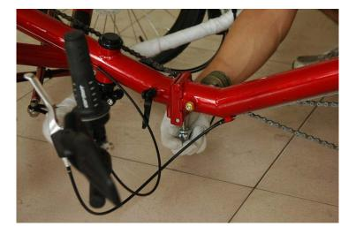
This lever is spring loaded (L&R). Pull the lever towards you to release the hinge pin.
