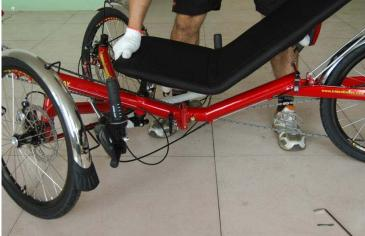
Loosen the quick release lever that holds the folding hinge and let it hang straight downward.
