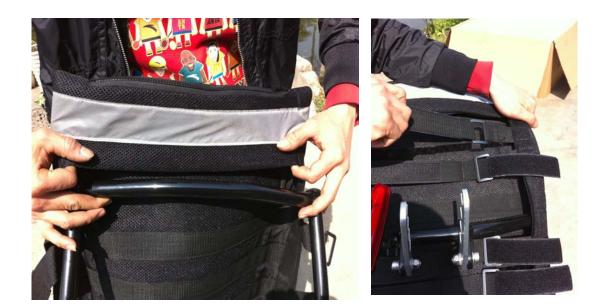
**Step 3:** Fasten the seat to the frame using the provided quick release skewers. It is easiest to do the bottom first. You have a choice of 3 seat heights . On the top you have four angle choices. Most people prefer to start with the more upright of the positions. Tighten quick release skewers fully.
