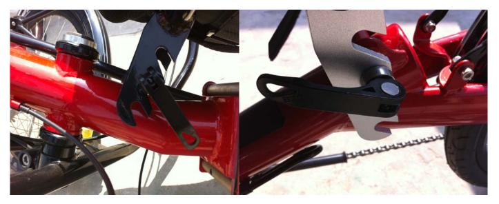
**Step 4:** Adjust boom length. The Boom is shipped turned at a 90 Degree angle. Loosen the boom and make sure the dreailleir post is perpendicular to the ground . Tighten a little so the boom does not rotate and attach the pedals - remember that the left pedal has reverse threads. Loosen boom bolts FULLY using a 6MM Hex Wrench. . Note: it is always important to fully loosen screws when adjusting boom- otherwise you will severely scratch the finish. It is also helpful if you put a
