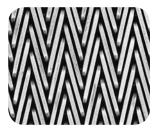
Compound balanced belting — this belt has right-and left-hand spirals fitted closely together for a smooth, dense weave. It is excellent for conveying very fine or small products, as well as unstable or top-heavy items. The compound balanced belt is used extensively in baking cookies, crackers, and snack foods. ■
