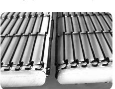
DuraHinge® belt after testing. Notice how the edges do not snag.
