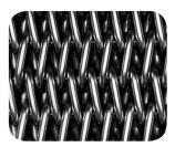
**Gratex belting** – similar to balanced belting except that the spirals are more closely wound, with a straight rod connector, producing a stronger, semi-closed mesh ideal for carrying small parts and heavy loads.
