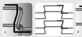
DuraHinge® Belt components (1) are designed with compound angles that hinge at each contact point, reducing stress and maintaining structural soundness. This design also enhances the true tracking nature of the belt.
