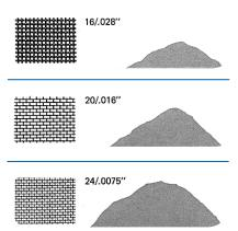
wire sizes provide longer life, but less screened material. Conversely, smaller diameter wires give greater capacity, but shorter service life. The illustrations above demonstrate the relationship between mesh, wire size, open area and screening capacity.
