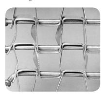
This welded-edge belt is suffering from necking-down, which occurs when the pickets compress on their rods, causing the rods to protrude along the edge. The belt was twisted out of shape when the protruding rods snagged along the edge of the conveyor.
