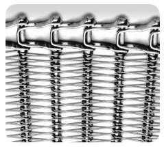
Cam-Grid® with mesh overlay.
