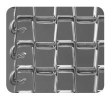
This belt has clinched edges. The connecting rods are curved back to grab the picket, draw it out to its fullest extension, and lock it securely in place. There is never any necking-down. Also, the clinched rods form a protective wear bar along the sides of the belt for strength and to discourage damage.
