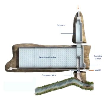
Figure 1 – Schematic representation of a storage basin.
