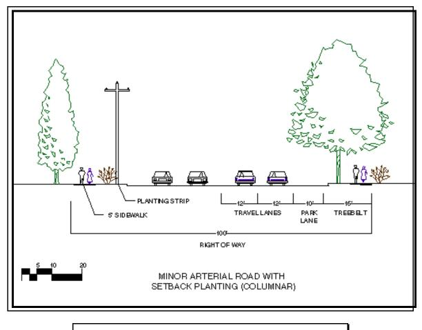
FIGURE 72 - Cross section of a minor arterial road with columnar tree species.
