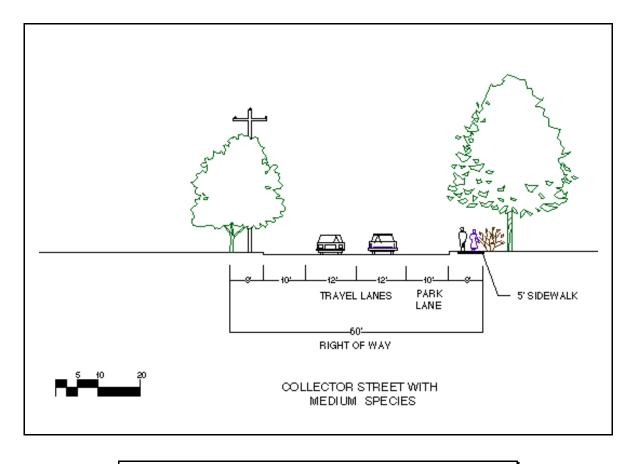
FIGURE 76 - Cross section of a collector street with smaller growing tree species.
