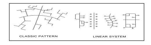
FIGURE 7 - Classic pattern and linear system of roadway layouts. *Source Harris/Dines, 1988.*
