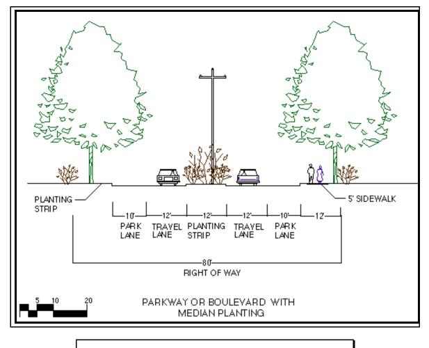
FIGURE 89 - Cross section of a boulevard street with shrub and small tree planting along center planting strip.
