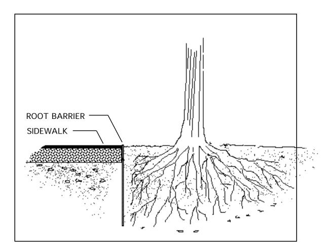
FIGURE 91 - Root barrier used to direct root growth downward away from physical infrastructure.
