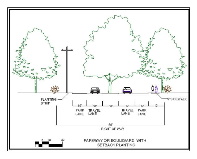
FIGURE 86 - Cross section of a boulevard street with setback planting.
