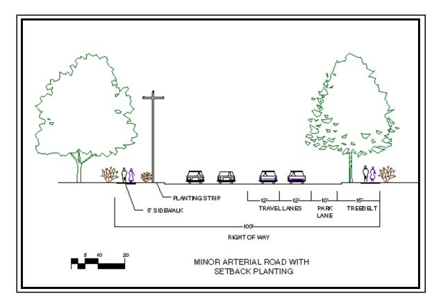
FIGURE 70 - Cross section of a minor arterial road with setback planting.
