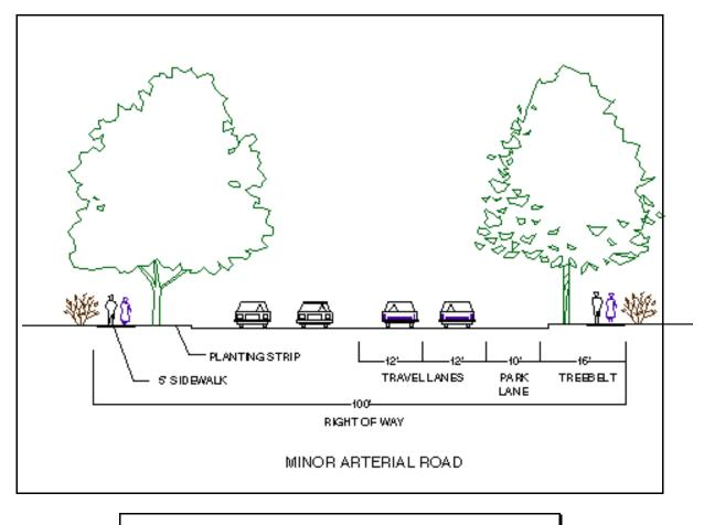
FIGURE 36 - Cross section of a minor arterial road.
