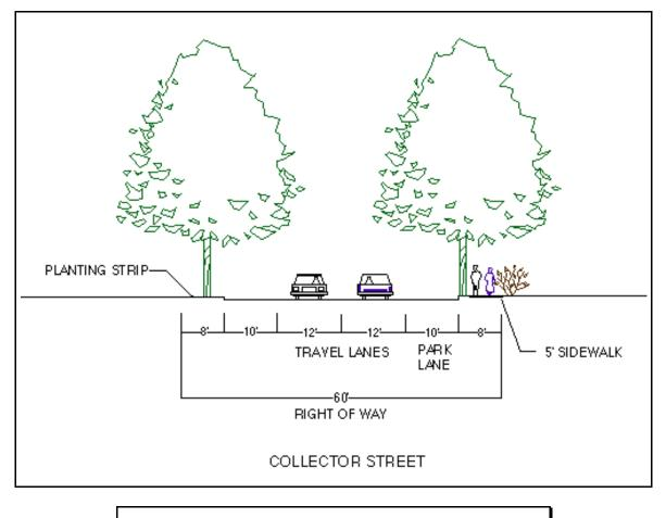
FIGURE 37 - Cross section of a collector street .
