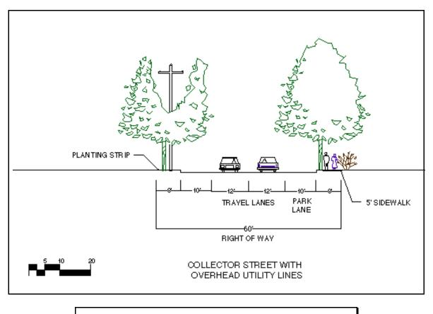
FIGURE 74 - Cross section of a collector street with overhead utility lines.
