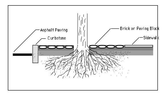
FIGURE 92 - Brick or pavers used to reduce potential damage to surrounding paving and allowing for improved permeability.
