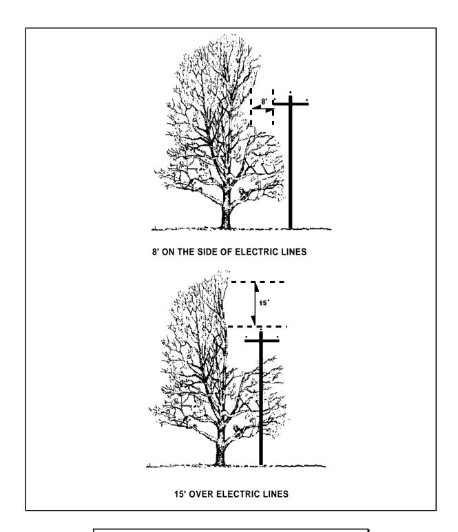
FIGURE 22 - Clearance distances from electric lines as required by Northeast Utilities.
