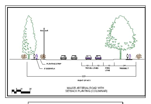
FIGURE 66 - Cross section of a major arterial road with columnar setback planting.
