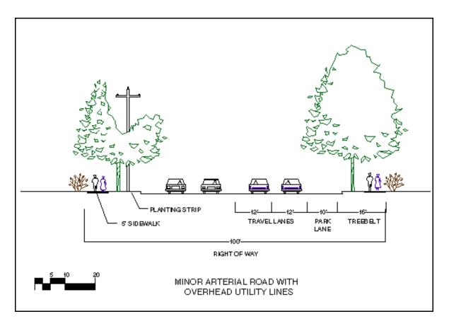
FIGURE 69 - Cross section of a minor arterial road with overhead utility lines.
