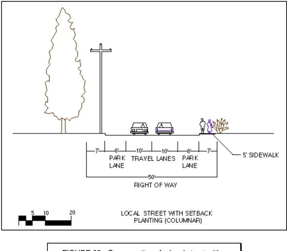
FIGURE 83 - Cross section of a local street with a columnar setback planting.
