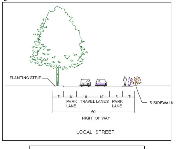
FIGURE 38 - Cross section of a local street .
