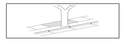
FIGURE 29 - Concrete sidewalk replaced with gravel or stone screenings. *Source Moll, 1986.*
