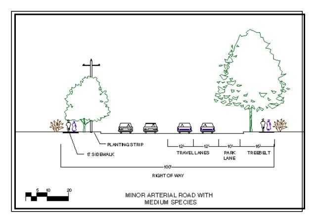
FIGURE 71 - Cross section of a minor arterial road with smaller tree species.
