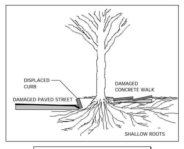
FIGURE 60 - Tree roots and damage to surface infrastructure.
