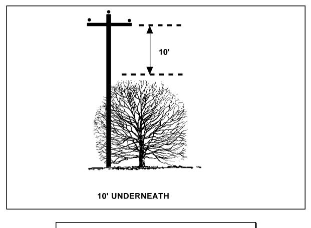
FIGURE 23 - Clearance distances from electric lines as required by Northeast Utilities.
