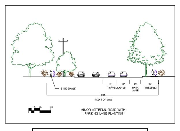
FIGURE 73 - Cross section of a minor arterial road with planting in parking lane.
