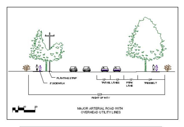
FIGURE 61 - Cross section of a major arterial street, including sidewalks on both sides of the street and planting strips.
