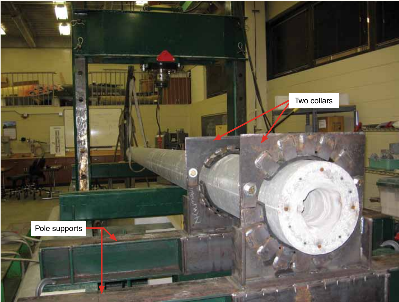
Figure 4. Details of pole end supports.
