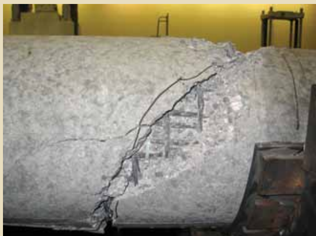
Figure 8. Concrete failure for poles confined with carbon-fiber-reinforced polymer (CFRP) grid.
