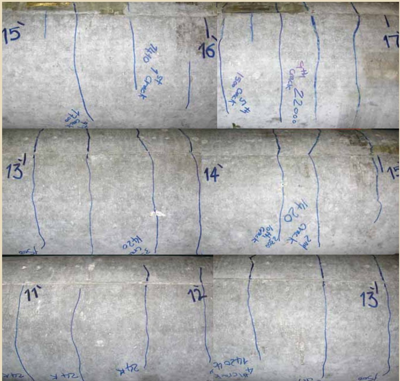
Figure 11. Cracking pattern for pole P03-12SS.
