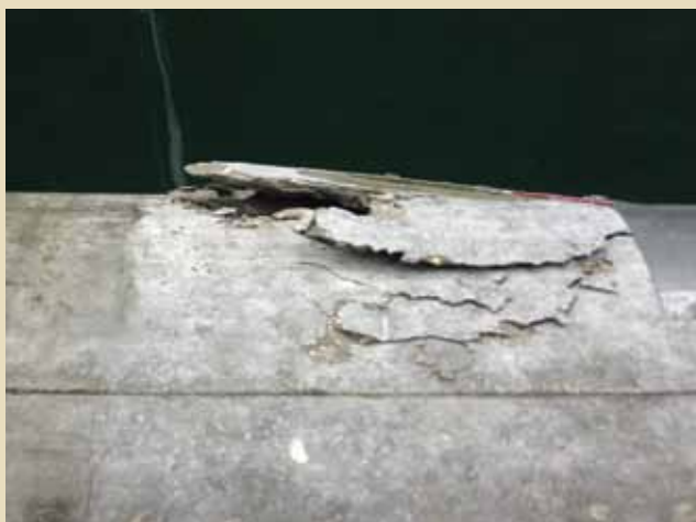
Figure 7. Concrete crushing at failure for poles confined with steel spirals.
