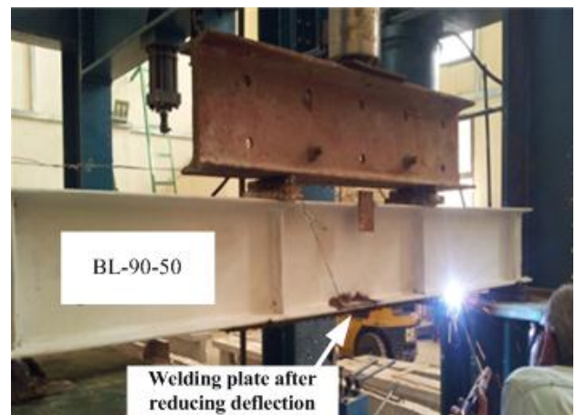
Photo2 Welding process during loading of specimen BL-90-50
