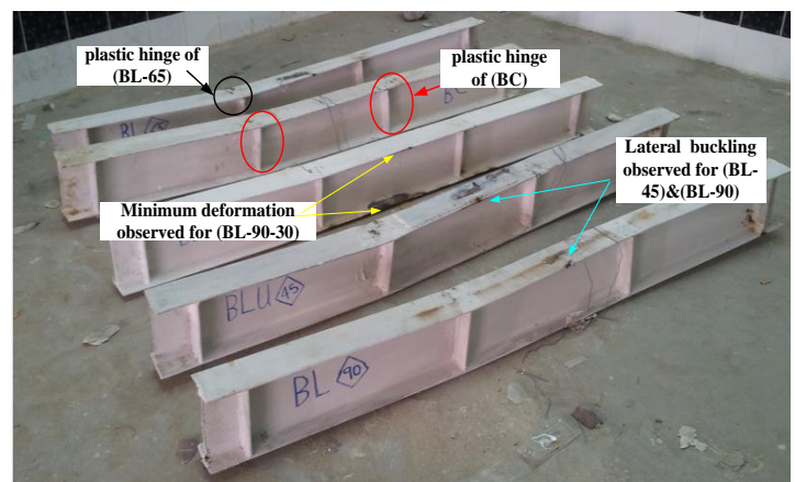
Photo 3 Failure modes of test specimens
