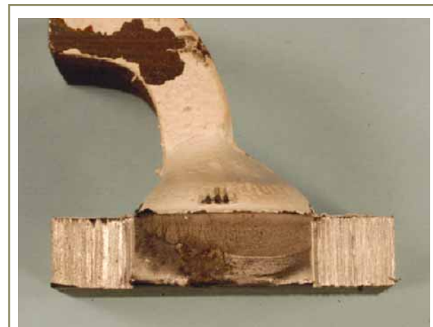
Figure 20 – The final shape of the fatigue crack initiated at the weld toe around the edge of the rectangular tube
