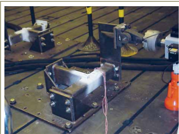
Figure 11 – The tubular welded joint subjected to torsion and bending load in the testing rig
