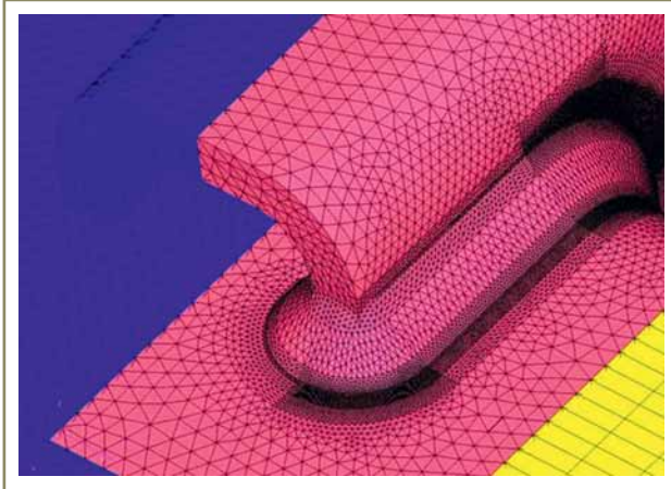
Figure 16 – Details of the 3D fine mesh FE model of the critical location
