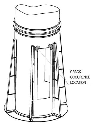
Figure 3. Chimney's root section
