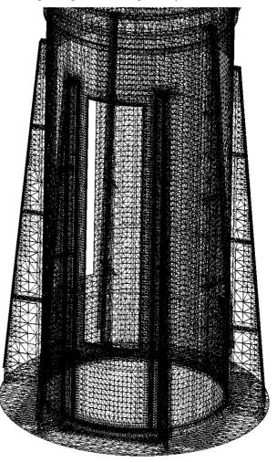
Figure 9. FEM Model of chimney's root section
