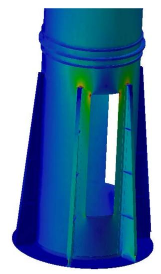
Figure 11. Uniaxial stress field on the chimney's root segment
