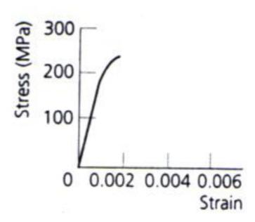
Above graph shows that gray cast iron exhibit less plastic region i.e it fractures just after elastic limit so it is a brittle material.
