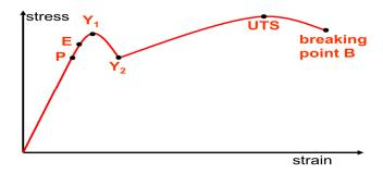
The above graph shows that the length of graph up to proportional limit (P) is a straight line which means that up to proportional limit stress is linearly proportional to strain.
