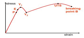
Among the common materials, only steel exhibits yield point. For annealed mild steel, upper yield point occurs at 260 MPa and lower yield point occurs at 230 MPa.
