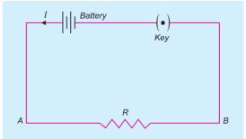
Battery is the source of energy or potential difference. Key is a safety device. The conductor carrying current is indicated by a resistance R. The direction of current indicated is that of conventional current. Instead of a battery, a dynamo or a battery eliminator can be used to create potential difference.
