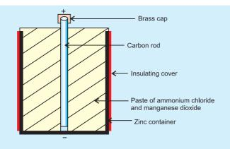
Dry cell produces 1.5 V potential difference between the carbon (+ ve) and zinc (– ve) terminals. Commercially these cells are produced by many companies and are used in torch, remote controls, etc., in day-to-day life.
