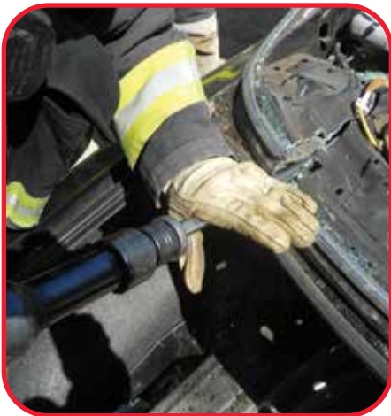
Cutting Rear Deck Lid
