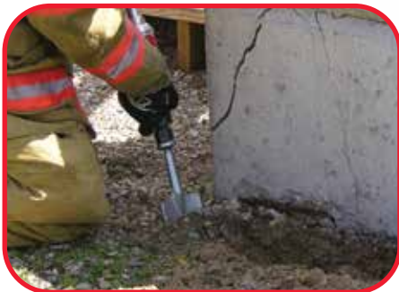
Spade bit for digging and trenching
