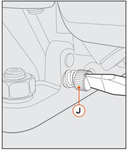
**NOTE:** If you have an engine vacuum gauge, set the idle screws to provide the highest and most steady manifold vacuum reading at idle.
