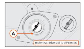
B) Install the Stromberg e-FIRE distributor, with its gasket (supplied) onto the front of the engine, engaging the distributor drive key into the offset slot on the end of the camshaft or cam drive adapter. Note that the drive key and camshaft slot MUST align to center the distributor on the mount. It is easier to install if you remove the
