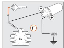
**Note:** Most early Ford 6 volt positive ground coils were ballast resisted. If possible connect the white module wire to the switched ignition side of the resistor (often located under the dashboard).
