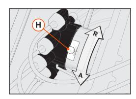
C) For advanced tuning, the Stromberg e-FIRE distributor also allows adjustment of the total mechanical advance and advance curve. Please visit the Stromberg Tech Center at www. stromberg-97.com for further advice.
