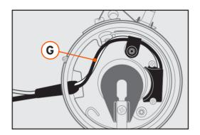
H) Terminals are supplied. Use standard auto wire - 20 gauge (1.5mm) 15 amp - to lengthen any wires. Crimp tightly or solder (best) the joints and insulate all connections. Do not pull on the wires causing them to tighten inside the distributor cap. The wires must allow movement of the timing adjustment plate, yet not interfere with any moving parts (see G).
