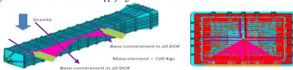
Fig.2 Container with 0.1Ksc internal pressure
