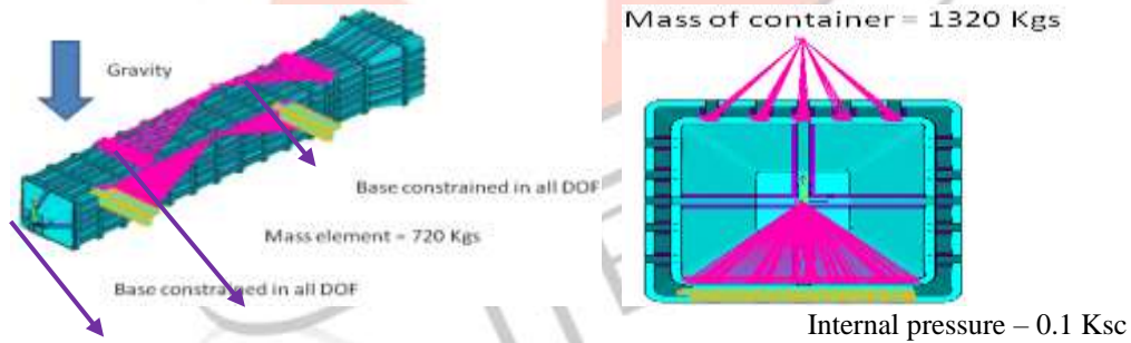
Fig.8 Container with internal pressure and stacking load
