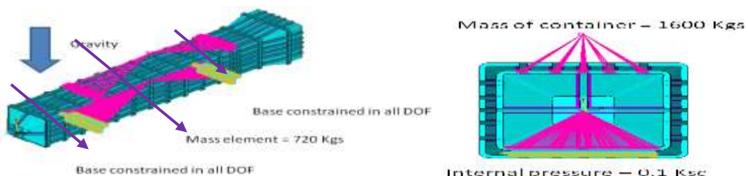
Fig.34 Container with internal pressure and stacking load
