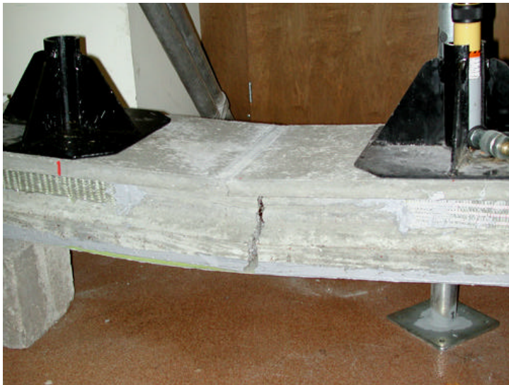
Figure 5 - Testing of concrete beam reinforced with fiber composites
