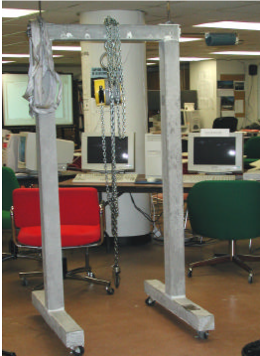
Figure 8 - Post-tensioned concrete crane used to lift heavy equipment in the lab.
