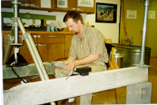
Figure 3 – Structural Analysis and Design student reading ultrasonic cover measurement
