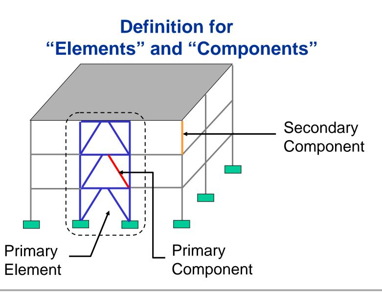
Primary elements or components are critical to the buildings ability to resist collapse
