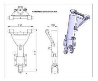
Fig.2 Assembled model of landing gear
