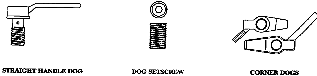
Figure 600-3.4. Straight Handle Bushing, Dog Setscrew, and Corner Dogs
