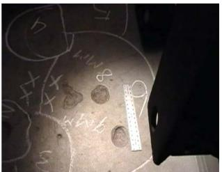
Photo 4- Bilge Plating-pitting corrosion
