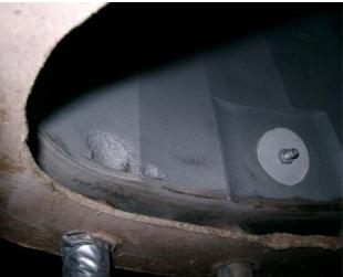
Photo 6-SSE Forging-galvanic corrosion
