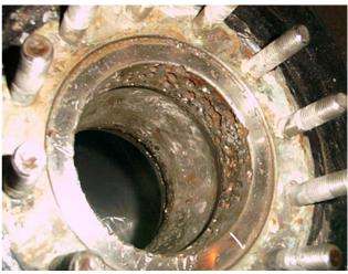
**Photo 2- Mechanical Hull Penetration**
