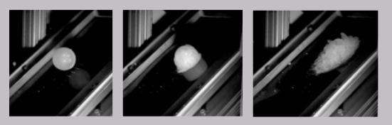
2.0 in. diameter ice impacting composite panel at 108 m/s (242 mph)
