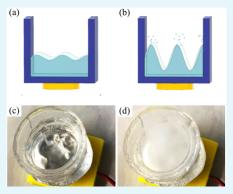
Fig. 1: Illustration and image of ultrasonic atomization
