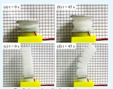
Fig. 2: Actuation of soft robotic structures
