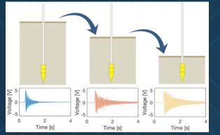
Fig. 1: The effect of scour on the piezo-rod's exposed length and subsequent output
