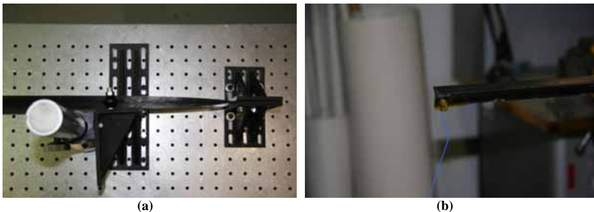
Figure 1. Preliminary static test. This test simulates the boundary conditions of the deployment mechanism. The boom is cantilevered horizontally. Analyzing Figure 1(a), the boom is clamped and fully compressed and then allowed to transition to a partially clamped/ semi-flared configuration.
