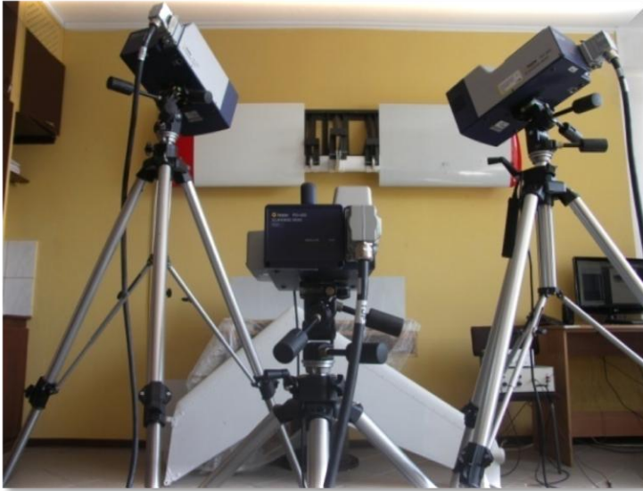
Guided waves monitoring by 3D laser scanning vibrometry
