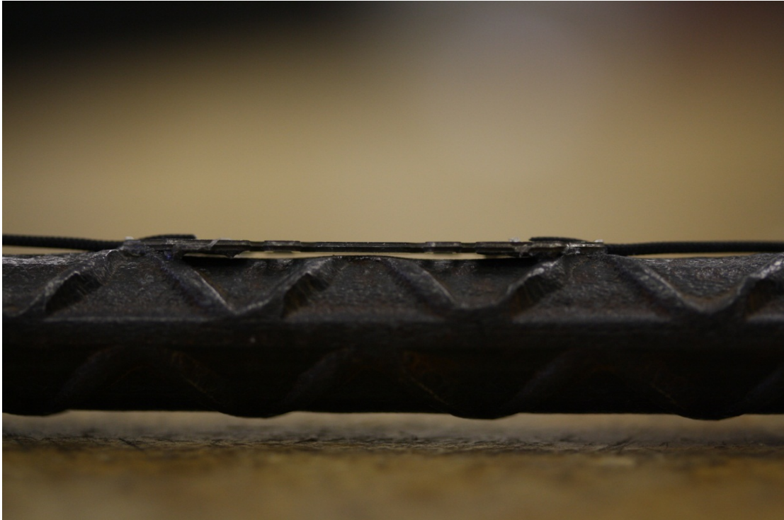
Figure 4-2: FOS attached with rebar
