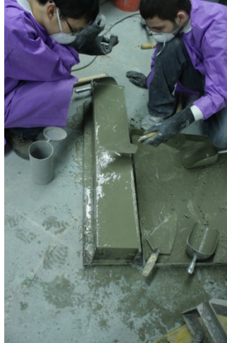
Figure 4-9: Casting of the RC beam
