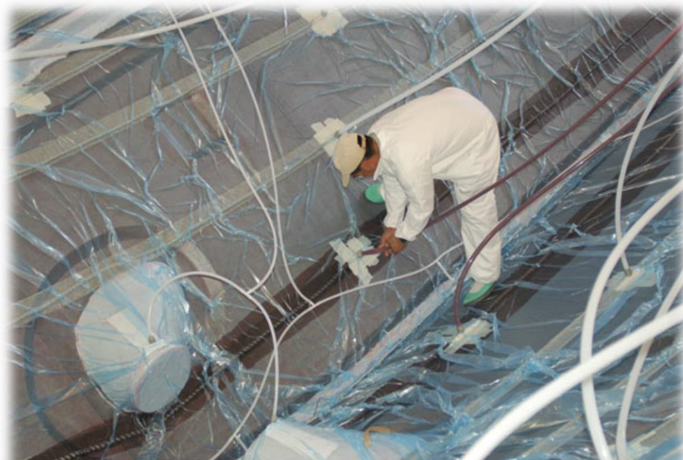
Tracking the flow of resin infusion is easy, just look for the dark areas to see the progress.
