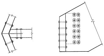
Figure 6 Bolted Rafter to Tie Beam Connection
