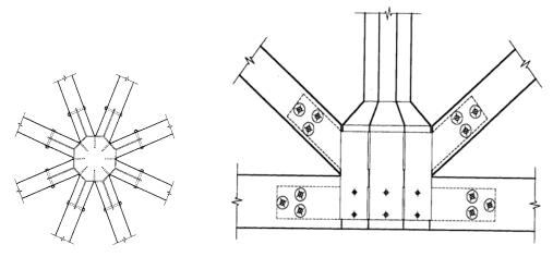
Figure 5 Multi-Member Bolted Joint
