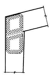
Figure 1 Nailed Plywood Gusset
