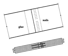
Figure 3 Nailed Timber Splice Joint
