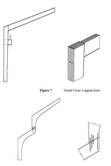
Figure 8 Epoxy Grouted Threaded Rods
