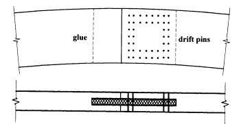
Figure 10 Timber & Drift Pin Connection
