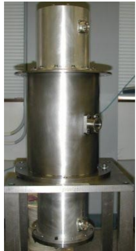
SW-18 conical magnetic bearing test rig.
