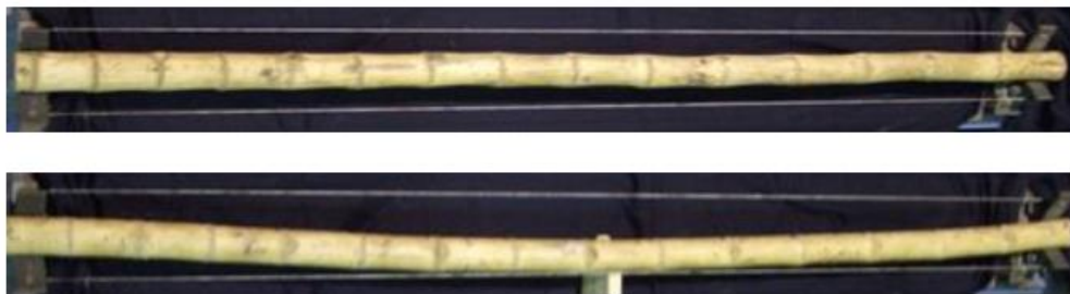
c) variation in straightness of Tre Gai culms of identical "batch" and storage conditions
