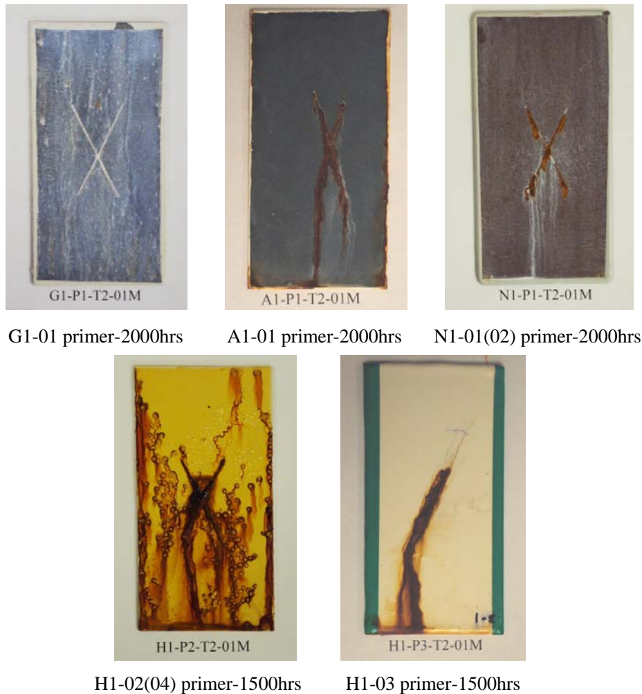
Figure 5.1 Primer Performance After 2000 (or 1500)-hour Salt Fog Test.
