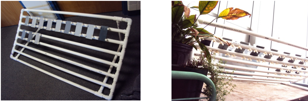
Figure 4.10 Atmospheric Exposure Testing Setup.
