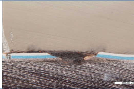
System N1-01 1500-hr & 3000-hr interface characterizations
