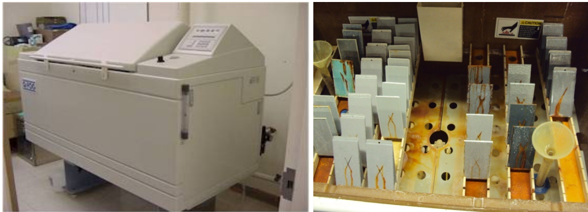
Figure 4.3 Salt Fog Test Setup.
