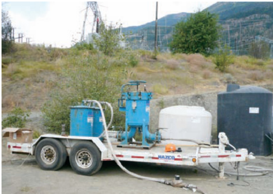
Figure 2.1 Photo of a Trailer-mounted Multi-stage Filter Rig for Removing Contaminants from Wash Water.
