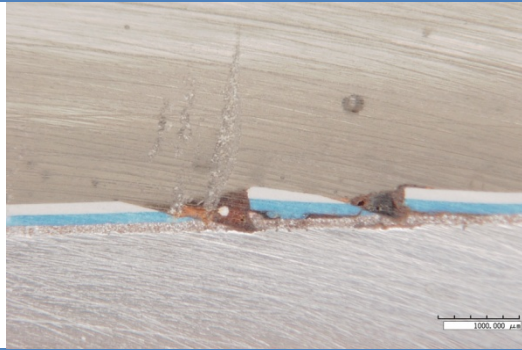
System N1-01 1500-hr & 3000-hr interface characterizations
