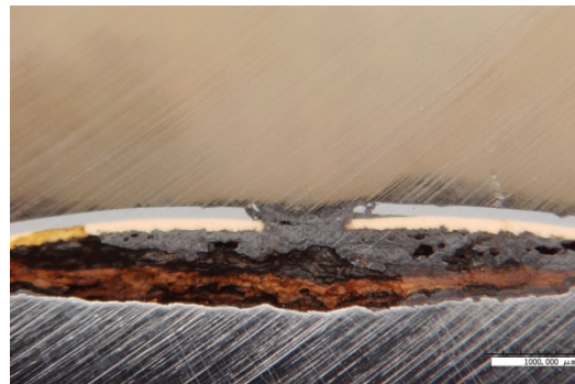
System H1-02 1500-hr & 3000-hr interface characterizations
