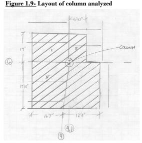
along column line G. However, these two factors were not taken into account in the spot check, resulting in a much smaller W 14x 82 column being selected as the initial size. Additionally, the area contributing to the column compression was not symmetrical. The dimensions of the tributary area for the column check are shown above in figure 1.9. Detailed calculations for the column check can be found in Appendix C.
