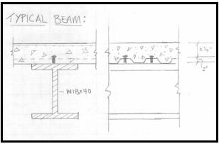
act with full composite strength allows the W-shape floor beams to develop a larger moment capacity, thus capable of spanning longer distances. The ability of a beam to span a longer distance results in further column spacing, allowing for flexibility in the floor plan which is a desirable trait in office building design. The concrete slab described above is shown in Figure 1.7 and is used as primary flooring system in all office spaces.
