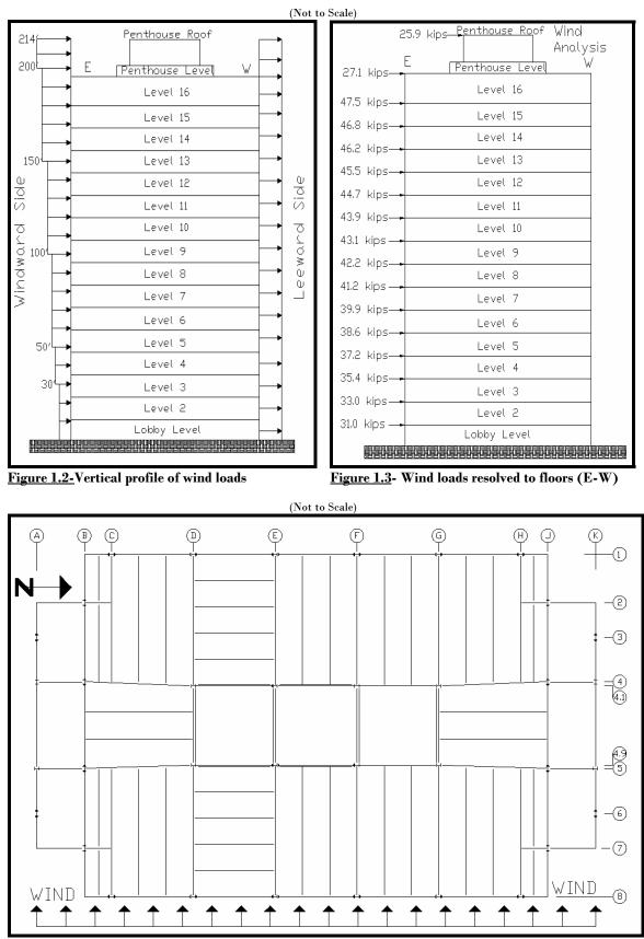
Figure 1.4- Wind force on E-W side of structure
