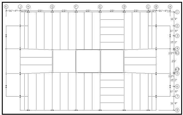
Figure 1.6- The typical framing plan found at levels 3 to 15
