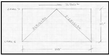
Figure 1.10-Analyzed braced frame on level 6
