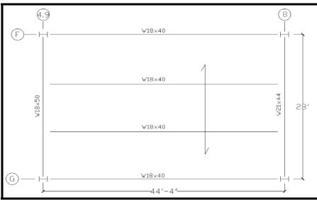
Figure 1.8- A typical bay from the 6<sup>th</sup> floor.
