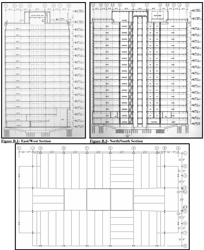
Figure B.3- Typical Framing Plan (Floors 3-15)
